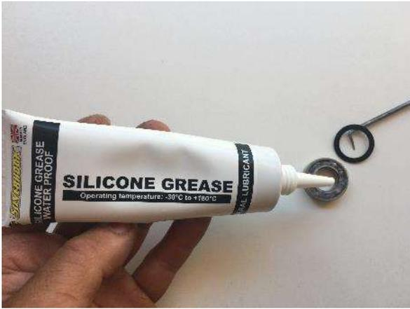
Next, pack the bearing with silicone grease and replace the seal. (Yes, I know you should not overpack a bearing, but this is not a high-speed application and therefore will not melt all the grease out and damage the bearing)
