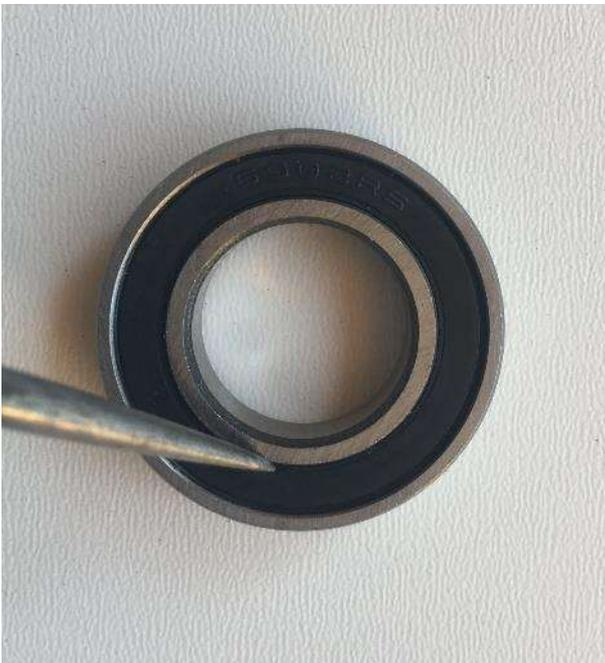
Remove the SES sprocket from your bike, remove the retaining circlip and press, drift or knock out the old bearing. Before fitting your new bearing remove the bearings outer seal using a pointy object like a scribe or a pin, careful not to damage the seal. (They are relatively easy to remove).
