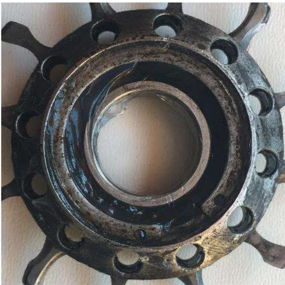
Press or drift the bearing back into your old SES sprocket and smear liberally with grease (this will need re-applying every month or so if you do a lot of wet or muddy riding)
