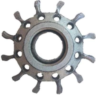
Here's one I took to the limit! Just to see what effect it would have on the chain and drive sprockets? The result: Really no discernible effect at all. The chain and other sprockets showed no sign of shortened life or excessive wear above and beyond normal.
